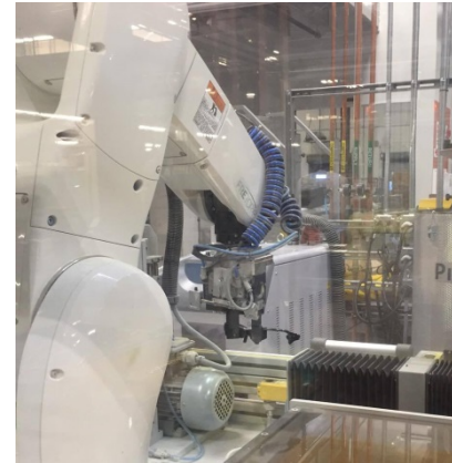
Denso Robot Arm performing frame pick-up
